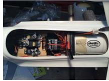
attach a tongue depressor to the top of the tank so the overall length is approx 8" long. Through the hole in the firewall will go the vent line directly to the muffler. Drill a hole in the side scallop about 1 1/2" behind the fuel nipple for your feed line. I like to run the feed line from the needle valve through the shutoff and between the mount and fuse side to the spray-bar. See Pic. The back of the tank goes up against the spar tube with a small bit of clearance for foam.
