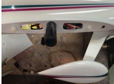
on top of the servo tray where the RX is all the way to the nose for the battery. Pack securely with foam so nothing shifts.
